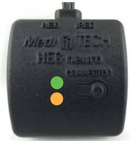
**Note:** If the connector flashes slowly, it searches for up to 30 seconds for the HEG neuro to which it connected the last time. If it does not find it, it starts flashing faster and searches for another HEG neuro in the vicinity.
