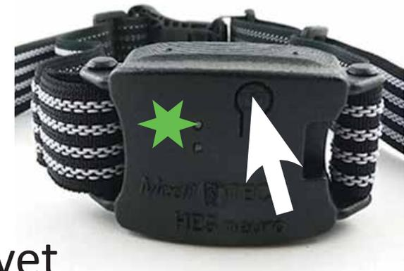
After a few seconds, the *HEG neuro* and the *connector* ,find each other'. You can recognize this by the fact that the upper lamp on the *connector* lights up continuously green. In addition, the lower lamp starts to glow orange.
