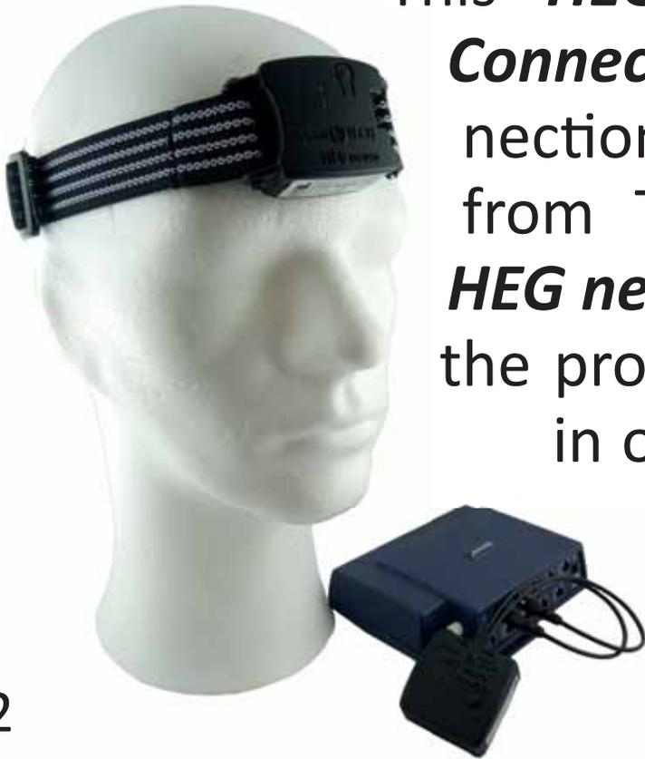
This ***HEG neuro Connector*** (referred to as ***Connector*** in this manual) establishes the connection between ***HEG neuro*** and a ***ProComp***<sup>®</sup> from Thought Technology. This allows the ***HEG neuro*** to also be integrated as a sensor in the professional work with ***BioGraph***<sup>®</sup> ***Infiniti*** in order to use the advantages of the HEG as a very easy-to-use method and to combine it with other parameters.
